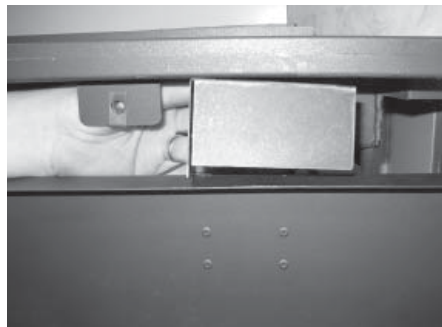
DC Spark Box Bracket Assembly partially removed.
